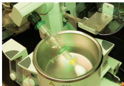
A variety of procedures and techniques are required for the preparation of biologically active compounds. The rotary evaporator (shown above) is commonly used at the very end to obtain the pure compound in a powder form.
